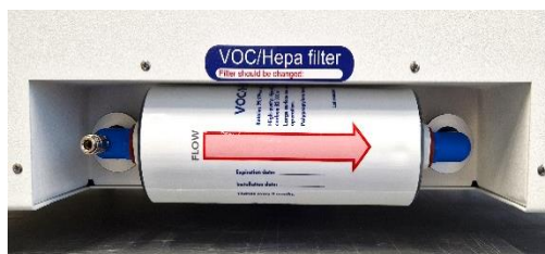
Figura 12.3 Filtru COV/HEPA corect instalat
